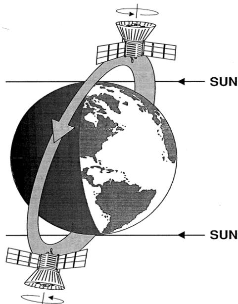
Fig. 1. Schematic view of COBE in orbit around the earth. The altitude at insertion was 900 km. The axis of rotation is at approximately  $90^\circ$  with respect to the direction to the sun. From Boggess et al. 1992.
