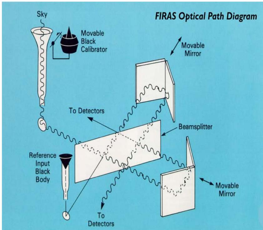
Fig. 4. The FIRAS optical path diagram. From [lambda.gsfc.nasa.gov/product/cobe](http://lambda.gsfc.nasa.gov/product/cobe)
