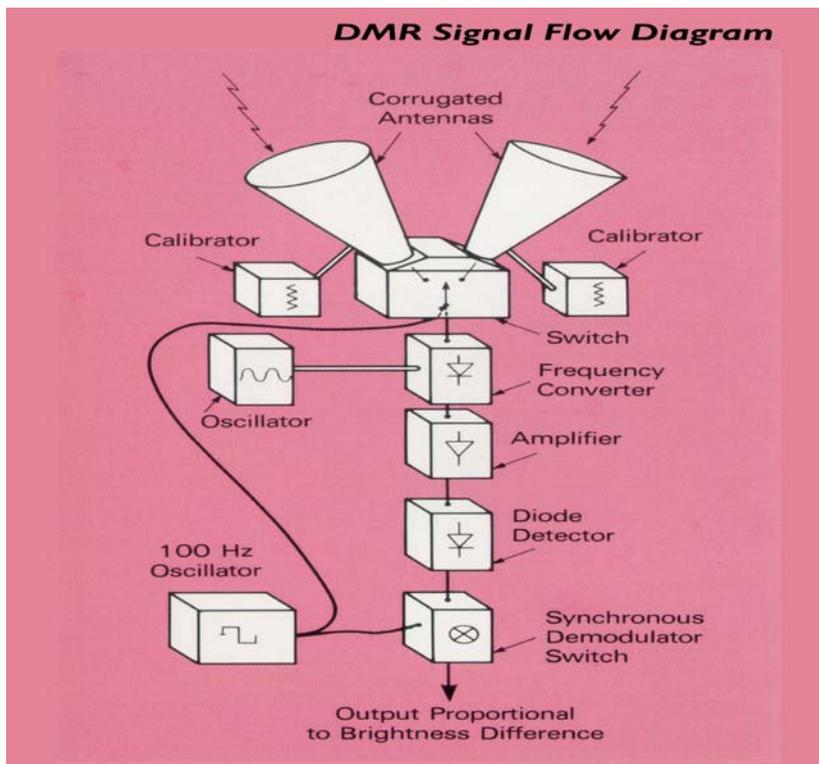
Fig. 3. The DMR signal flow diagram. There were six differential radiometers, two for each wavelength. Each pair had detectors separated by  $60^\circ$ . From [lambda.gsfc.nasa.gov/product/cobe](http://lambda.gsfc.nasa.gov/product/cobe)
