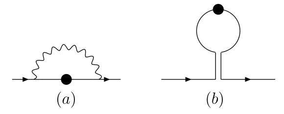
Self energy contributions to the quark propagator: (a) gluonic correction from the continuous dimensions, (b) tadpole correction due to hops in the lattice directions.
