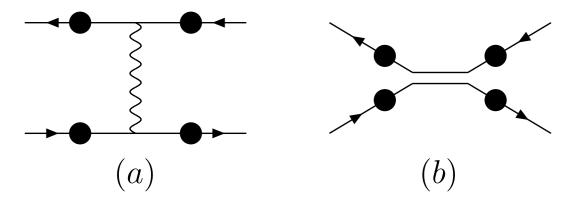
The interactions between quark and anti-quark in a meson: (a) gluon exchange in the continuous dimensions, (b) colour singlet hops in the lattice directions.
